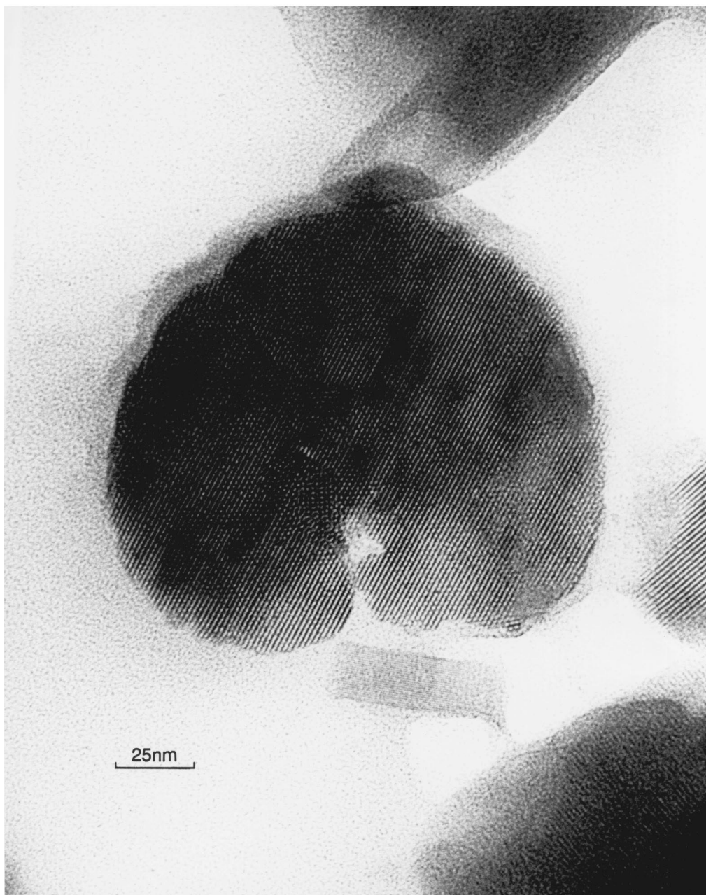
Fig. 2. Transmission electron microscopy image of Pt clusters supported in zeolite LTL [7].
